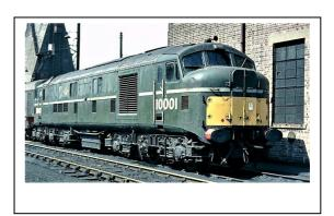
LMS No. 10000 and 10001 were the first mainline diesel locomotives built in Great Britain. They were built in association with English Electric by the London, Midland and Scottish Railway at its Derby Works, using an English Electric 1600 hp diesel engine, generator and electrics.
