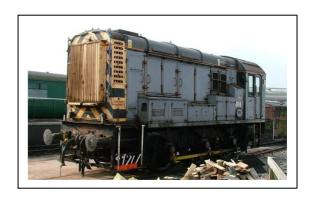
The British Rail Class 08 is a class of diesel-electric shunting locomotive. The Pioneer Class 08 No. D3000 (currently preserved at the Heritage Shunters Trust based at Peak Rail) was built in 1952 although it did not enter service until 1953. Production continued until 1962; 996 locomotives were produced, making it the most numerous of all British locomotive classes.
